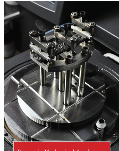
Dynamic Mechanical Analyzer measures flexibility and toughness
